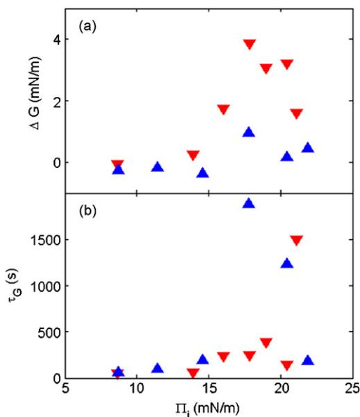
Fig. 6. The amplitude (a) and timescale (b) of the shear modulus relaxation, obtained by fitting the relaxation with a simple exponential decay function. Only  $\beta$ -lactoglobulin pH 8.3 ( $\blacktriangledown$ ) and pH 6.0 ( $\blacktriangle$ ) are shown since for  $\beta$ -casein this shear relaxation is negligible throughout the investigated range.
