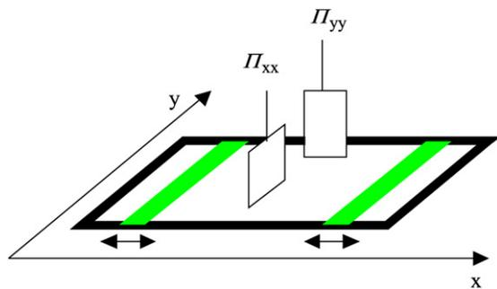
Fig. 1. Diagram of the Langmuir trough setup with symmetric compression barriers confining the monolayer film to the central area of the trough. Two pressure sensors record the surface pressure at the same time. The two sensors are maintained at  $90^\circ$ , and record pressures  $\Pi_{xx}$  and  $\Pi_{yy}$ , as indicated.
