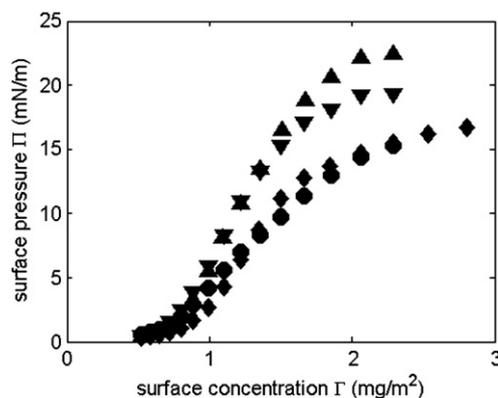
Fig. 2. Equilibrium surface pressure as a function of the surface concentration for the four systems studied in this work:  $\beta$ -lactoglobulin pH 8.3 ( $\blacktriangledown$ ) and pH 6.0 ( $\blacktriangle$ ), and  $\beta$ -casein pH 8.3 ( $\bullet$ ) and pH 6.0 ( $\blacklozenge$ ).
