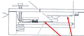
Measure separation via interferometry. Use springs of different stiffness. Determine when attraction is sufficient to cause surfaces to jump together into contact.
