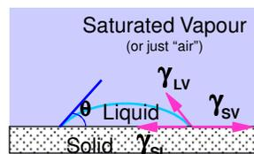
Balancing forces (recall surface energy  $\equiv$  surface tension per unit length) at the contact line, where the solid, liquid and vapour phases meet
