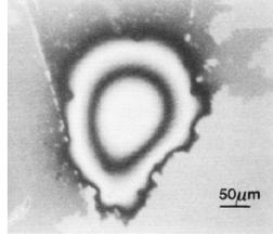
Interference fringes can be used to monitor drop shape/thickness, and the way in which the droplet spreads. The dynamics of spreading can thus be followed in real time.
