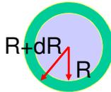
Work done is  $\Delta p \cdot 4\pi R^2 dR$ , where  $\Delta p$  is the difference in internal and external pressure, i.e. is the pressure driving the expansion.
