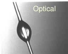
Water droplets on a cellulose fibre.
