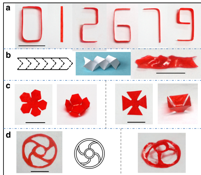
Fig. 3 Solvent-induced shape programming by origami and kirigami. a Digital numbers formed by origami from a strip. Scale bars: 1 cm. b A crease structure obtained by Miura-origami. (left panel: folding along with the dotted line; middle panel: illustration of a crease structure; right panel: the obtained crease-structure.) Scale bars: 1 cm. c Assembled 3D structures by origami and kirigami. Scale bars: 1 cm. d A steering-wheel-like 3D shape obtained by kirigami. (left panel: a cut flat steering-wheel-like film; right panel: the obtained 3D structure.) Scale bars: 1 cm
