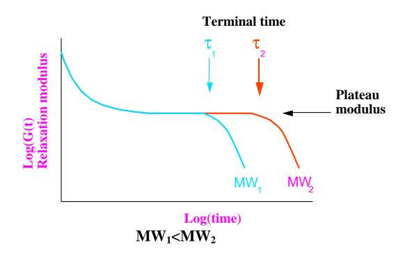
Once the chain has completely escaped no further resistance to deformation, and hence G drops.
