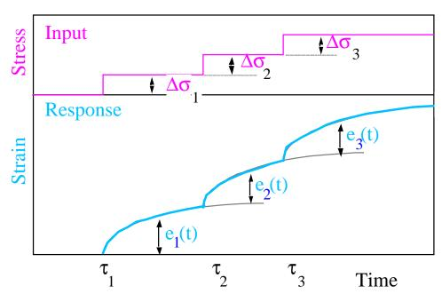
In general, for a creep experiment, increments of stress  $d\sigma$  at times  $t_n$
