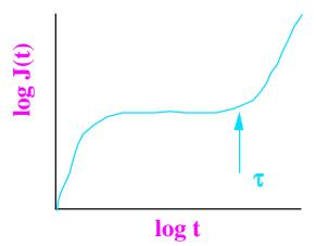
As with rubbers, for which we identified a plateau modulus inversely related to  $M_x$  (the MW between crosslinks), for entangled polymers we can find an equivalent quantity –  $M_e$ , the MW between entanglements – from the value of the plateau modulus.
