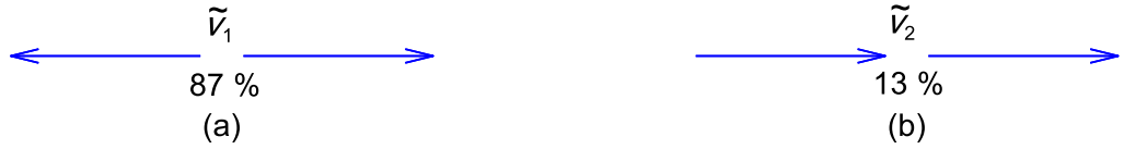
Figure 3. In the simplest case of two beads, oscillating on axis (i.e. (\theta_1, \theta_2) = (0, 0) ) the two normal modes of oscillations \tilde{v}_1, \tilde{v}_2 are simply antiphase motion (a) and in-phase motion (b). The geometry of the modes is illustrated by the vector pairs \tilde{v}_1, \tilde{v}_2 ; the eigenvectors are labeled from 1, \dots, N (in this case N = 2 ) in the order of decreasing relaxation timescale, and this convention is followed throughout this paper. The percentage indicates the fractional amplitude observed experimentally from the decomposition of the steady-state solution onto the normal modes.
